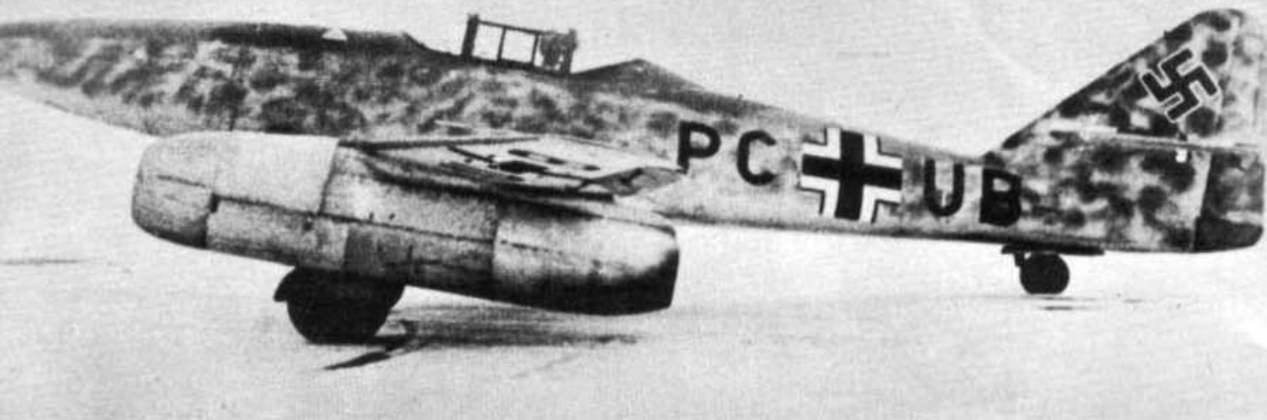
The Me 262V2 (PC+UB) with early model Jumo turbojets, single piece ailerons with external mass balances and elevators fitted with hoop mass balances. Note sharply raked mainwheel fairing doors and lack of mass balances on the rudder and trim tab.
