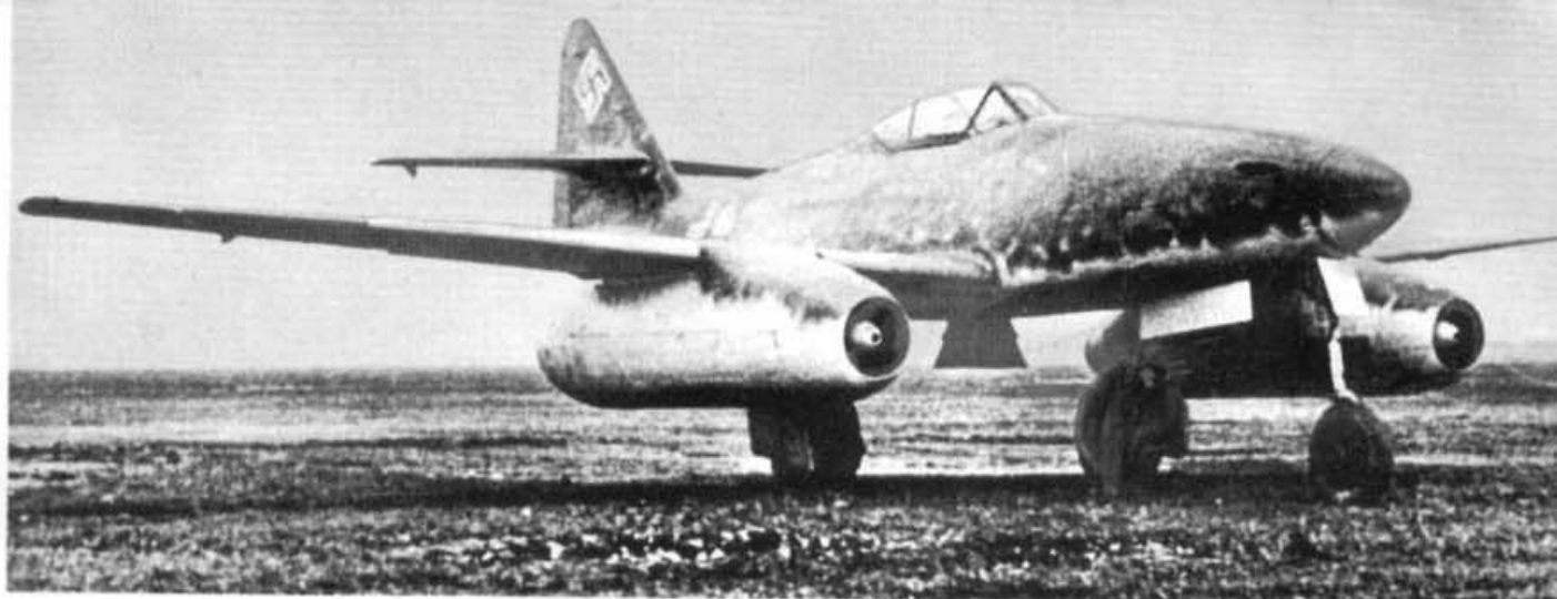
Another Me 262A-2a minus bomb racks and showing the upper guns deleted, the recesses being covered by doped fabric.
