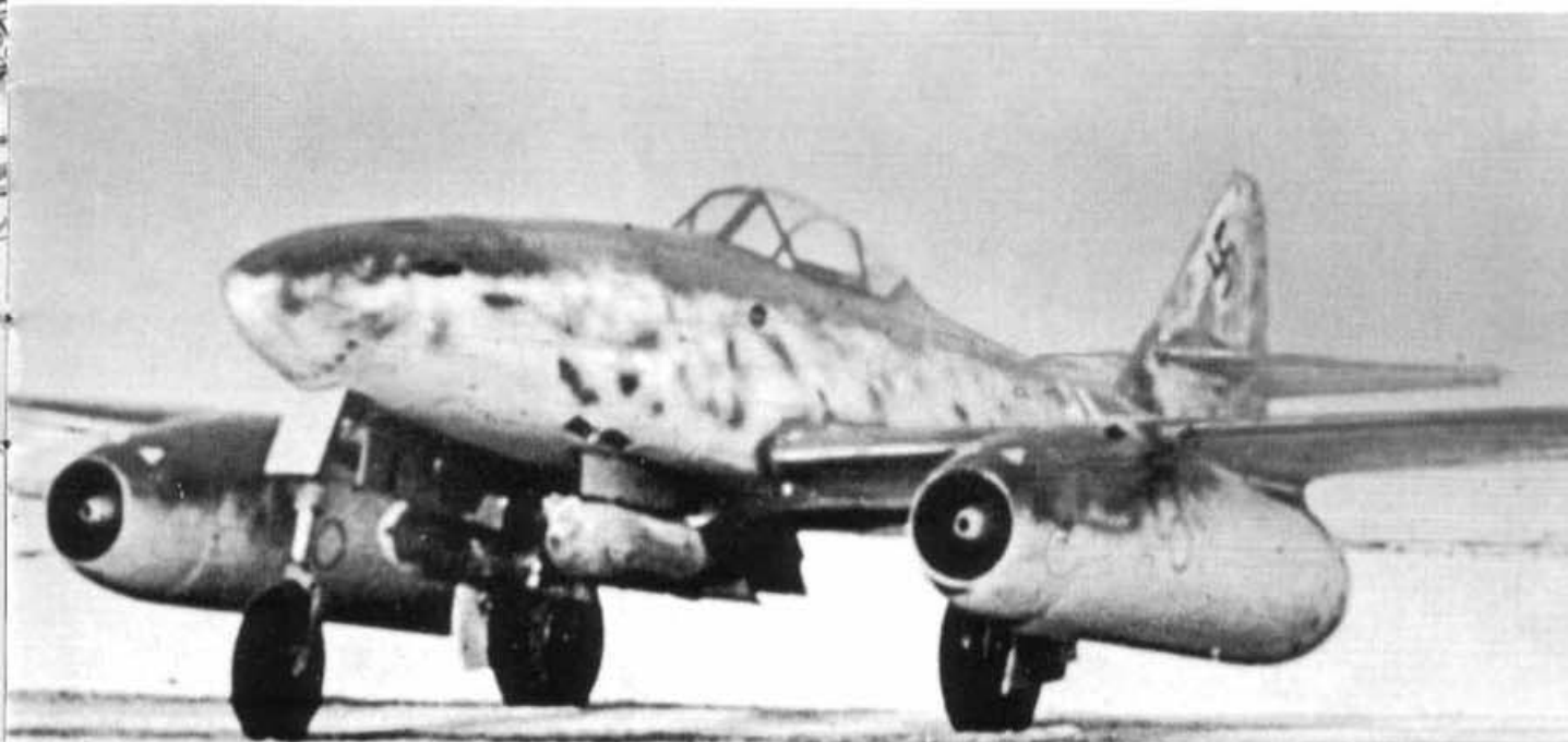
An Me 262A-2a with full war load of two 250 kg. bombs and carrying the full complement of four cannon.
