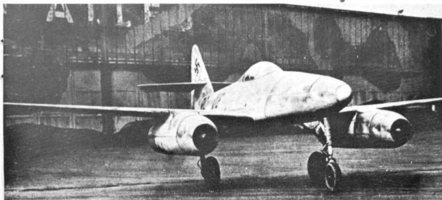
Another view of the Me 262V5 showing the prototype nosewheel installation.
