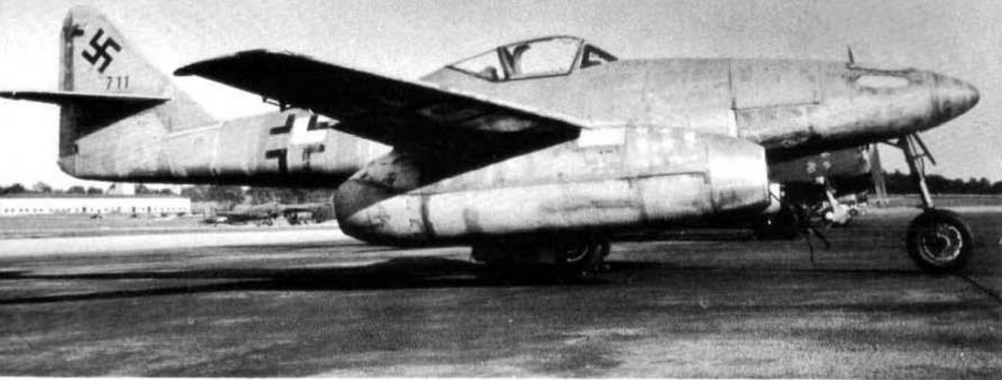
An Me 262A-2a Werk.Nr.111711 in natural metal finish. Despite the lack of bomb racks this WAS a bomber variant and details of its capture will be found in Part II of this work.
