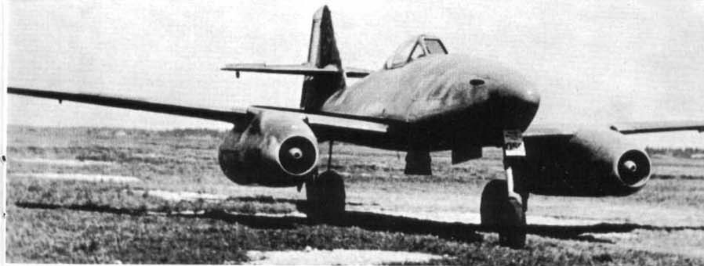
An Me 262A-2a minus bomb racks and with the upper cannon deleted.
