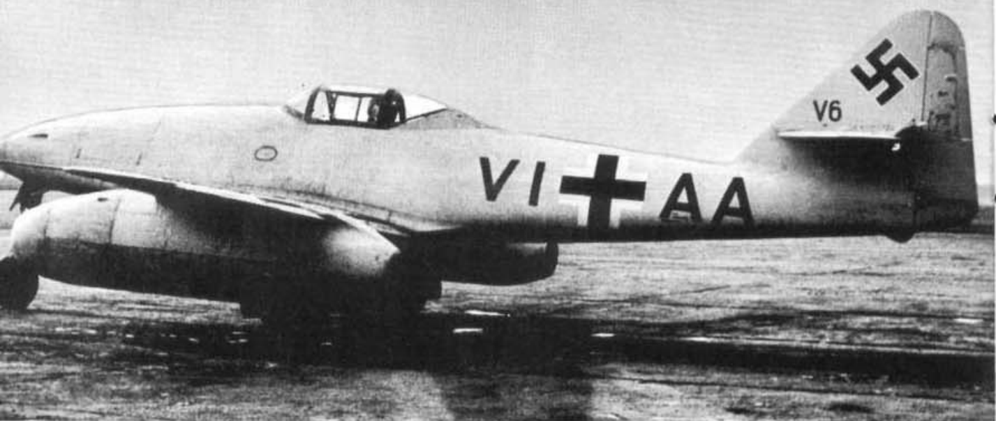
The Me 262V6 (VI+AA) with the late model Jumo turbojets of the production series aircraft showing the revised cowling panels. Both rudder and trim tab have mass balances. Note cannon ports and the repositioned hydraulic filler point.
