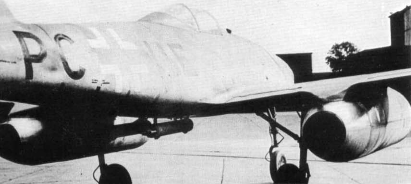
The Me 262V5 (PC+UE) after modification to the tricycle undercarriage layout. The undercarriage was fixed in the down position, the main wheel centre doors were locked shut and the oleo fairings removed to reduce the drag as much as possible. Two Borsig rockets are visible beneath the fuselage. The original shape of the trailing edge-engine fillet fairings is clearly shown.
